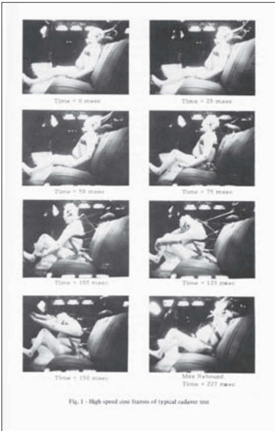
FIGURE 59 Crash test with cadaver. Proceedings of Nineteenth Stapp Car Crash Conference (1975) , p. 9.
