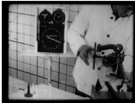
Figure 2 A typical shot from one of Gilbreth’s motion study films. Note the chronometer, the grid, and the camera angle THE QUEST OF THE ONE BEST WAY (USA 1968)
