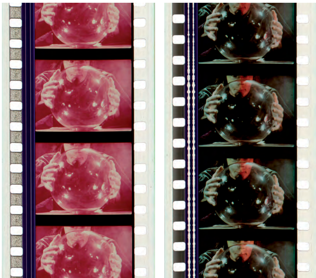
Figs 13 & 14: Images before and after restoration of the color-faded film Musica eterna 1452-1952 (Netherlands, 1951 - courtesy of Philips and EYE Film Institute Netherlands)
