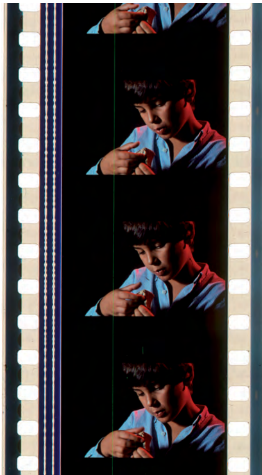
Fig. 2: Example of color line scratch on a film print of Romance de Valentia (Sonia Herman Dolz, Netherlands, 1993 – courtesy of EYE Film Institute Netherlands)
