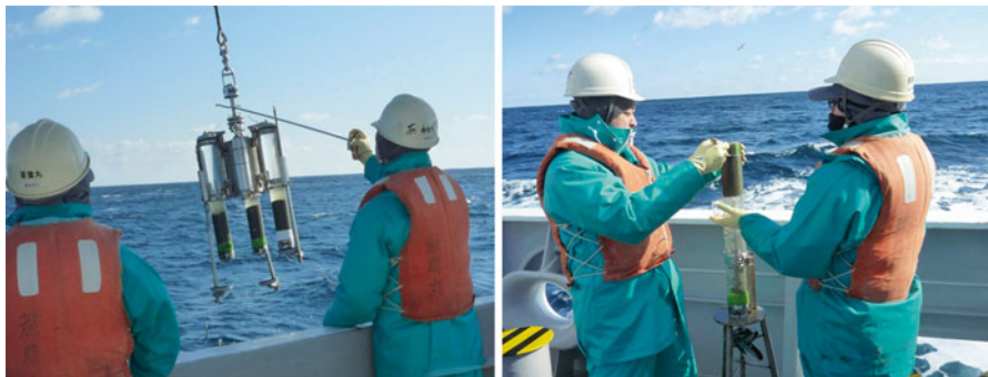
Fig. 4.2 Photographs of collecting sea sediment by a tube-type core sampler
