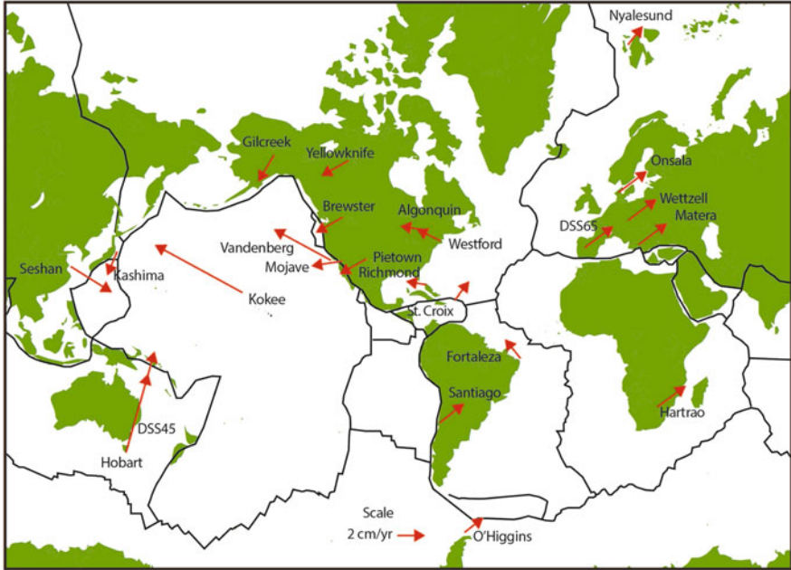
Fig. 1.22 Tectonic plate motions measured with VLBI. A VLBI station is located at the foot of each vector and labeled by the station name. The sum of the motion vectors is constrained to be zero. The largest motion is for the Kokee site in Hawaii, about 8 \text{ cm yr}^{-1} . Plate boundaries, established by other techniques, are shown by the jagged lines. From Whitney et al. (2014). Reprinted with permission courtesy of and © MIT Lincoln Laboratory, Lexington, MA.
