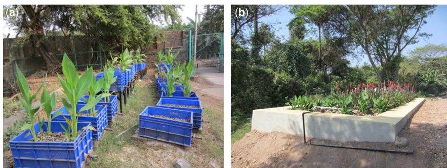
Figure 9.2 Laboratory CW-reactors and pilot-scale CW facility used in the research on IIT Bombay Campus, Mumbai. (a) Laboratory CW-reactors, (b) Pilot-scale HSSF-CW at IIT Bombay Campus.
