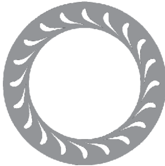
Figure 5. The 3-D design of nozzle in turbine.
