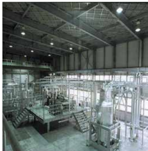
Figure 2. 4.5-kW experimental equipment of OTEC using the Uehara cycle (Saga Univ).
