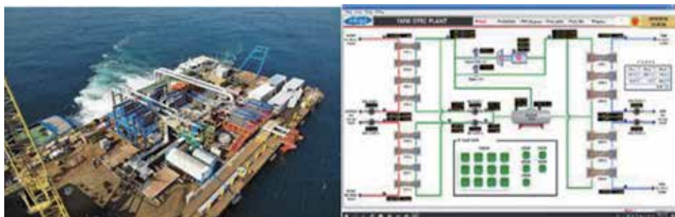
Figure 17. Operation scene of barge-mounted 1 MW OTEC plant (L) and monitoring system (R).
