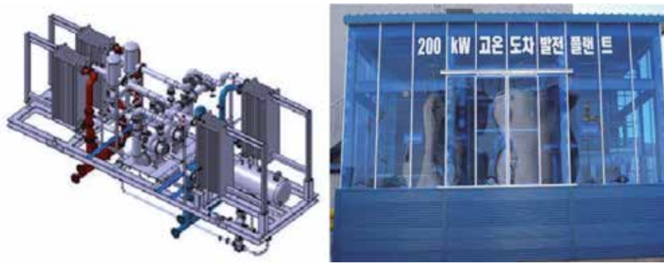
Figure 3. A 200-kW HOTEC plant using 80°C heat source (KRISO): 3D graphic (left) and photographic image (right).
