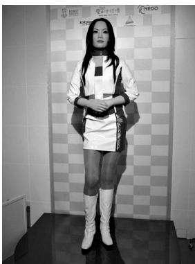
Figure 2: The “gynoid” robot ACTROID-DER, developed by KOKORO Inc. for customer service, appeared in the 2005 Expo Aichi, Japan. The robot responds to commands in Japanese, Chinese, Korean, and English. 4
