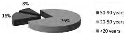
Figure 4. Age structure of water pipe network.
