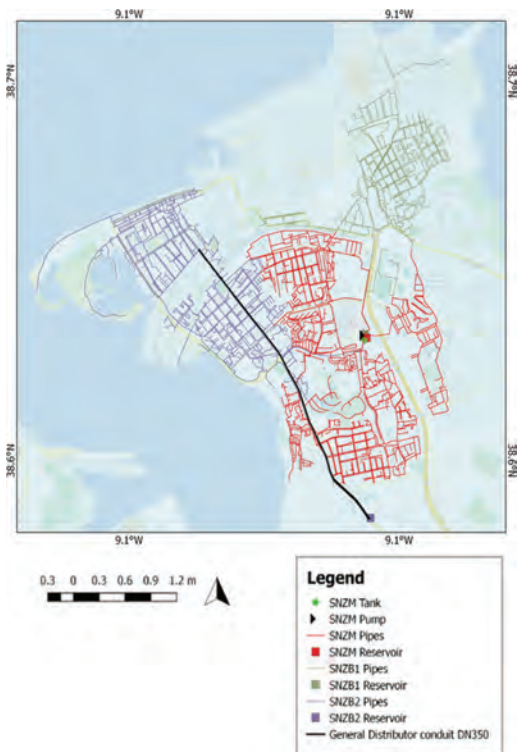
Figure 2. Barreiro Study Site Pipe network and Reservoir.
