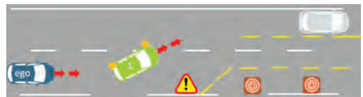
Figure 5. Evolution of the scenario: An event occurs consisting on the presence of the WZ.
