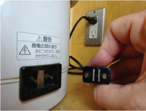
Figure 1. Japanese safety related construction: Easy detachable connection to avoid electric cable damage in case of force effect (e.g. caused by earthquake and involved vibrations).
