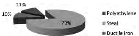
Figure 3. Material structure of water pipe network.
