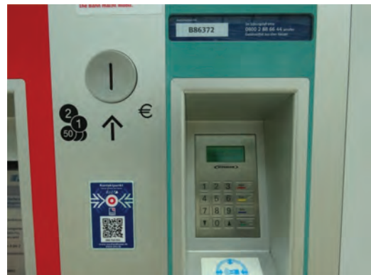
Figure 3. Ticket machine: Standard solution, focus: single coin slot regarding paying by coins, procedure is one-by-one.
