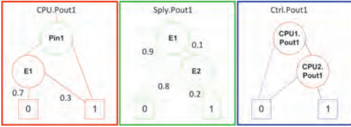
Figure 2. BDD fragments for the example CFT: main component (left) and subcomponent C1 (right).
