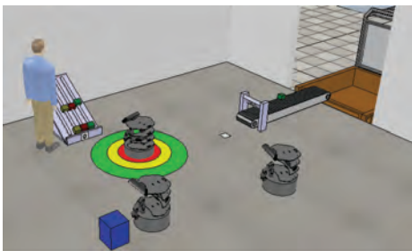
Figure 1. Illustration of robots in the warehouse and the dynamic safety fields. The blue cube is the recharging station, the small boxes in red, green and brown are products on the shelf, and a white square on the floor next to the conveyor belt is a way-point. The green (clear), yellow (warning) and red (critical) circles are the safety zones around the robot.
