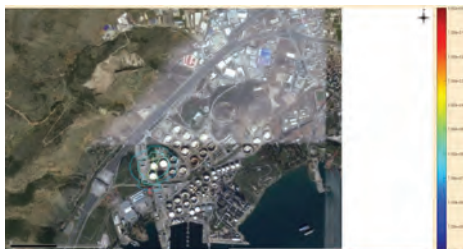
Figure 3. Isorisk curves and consequences zone for plant damage state (b), Continuous release.
