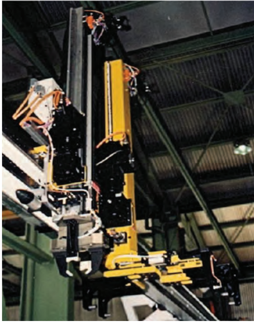
Figure 1. Robot arm used for handling of heavy parts, from DGUV (2012).
