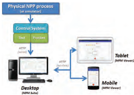
Figure 10. Data server connectivity.
