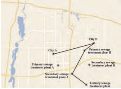
Figure 6. The original design of the sewage system.
