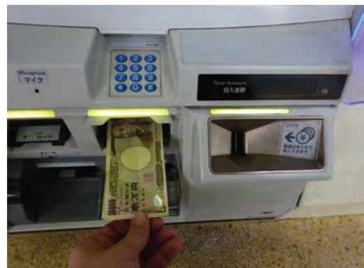
Figure 4. Ticket machine: Optimised solution based on Japanese Engineering. Focus: Parallel paying (e.g. coin slot hopper form).
