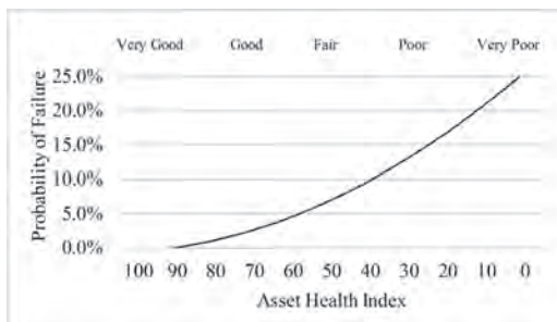
Figure 2. Asset health index ranges and the relationship with the probability of failure.
