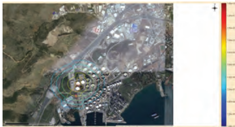
Figure 2. Isorisk curves and consequences zone for plant damage state (a), Instantaneous release.
