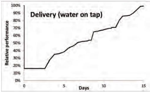
Figure 3. A simulation of the delivery to tap after the event using analytical models and EPANET modelling using fragilities of each pipe.
