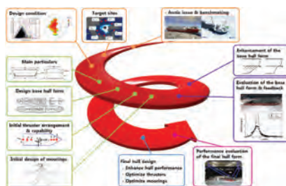
Figure 3. Design procedure (design spiral) of the offshore plant structure with the DP and mooring system in Arctic sea.
