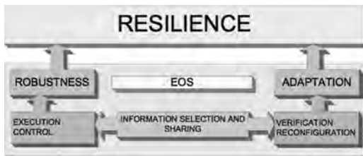
Figure 3. The Model of Resilience in Situation (MRS) identifies five functions of the Emergency Operating System (EOS): ‘Execution’ and ‘Control’ ensure the system’s robustness, ‘Verification’ and ‘Reconfiguration’ the system’s adaptation, while ‘Information selection and sharing’ is a cross-cutting function enabling the other functions.
