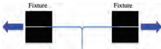
Figure 5. Specimen installation method.
