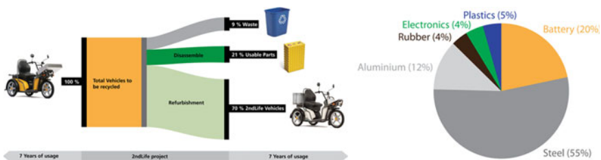
Fig. 13 Majority of the KYBURZ DXPs are refurbished, and those which are recycled result in good yields
