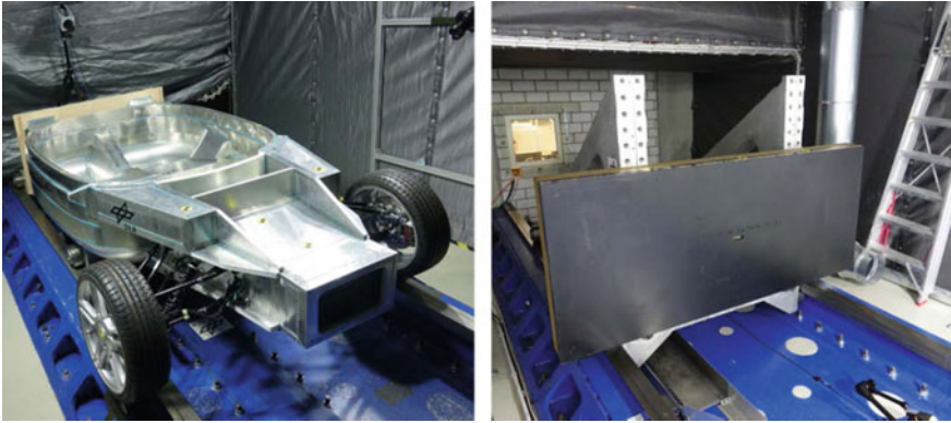
Fig. 6 Left: Experimental set-up for the frontal crash test, with sled 2 fixed; Right: sled 1 in motion
