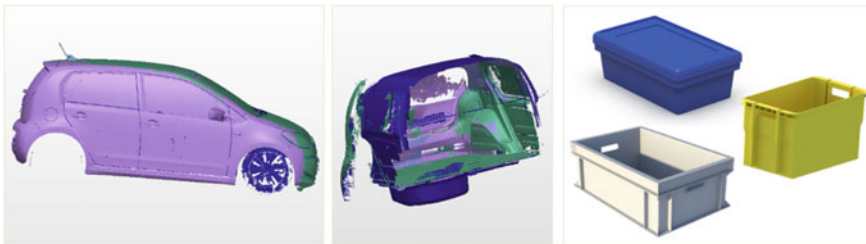
Fig. 3 LIDAR-Scan of the VW e-up! load-up! ; left: exterior; centre: cargo compartment; right: pharmaceutical cargo containers, “ Postbehälter Typ 2 ” and VDA/Euronorm
