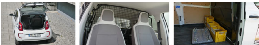
Fig. 2 Volkswagen e-up! load-up! with cargo compartment (left and middle) and a typical example of parcel and mail transport with an internal combustion-engine-powered transporter (right)
