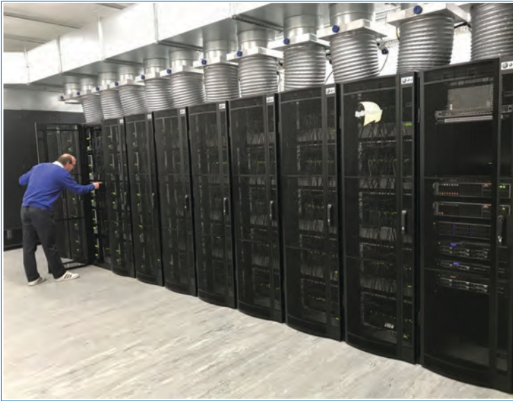
Figure 3.20. SpiNNaker1M : SpiNNaker million-core machine.
