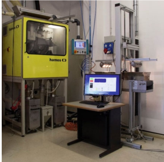
Fig. 5.4 Prototype for feed-forward control strategies: HSI workstation (right) and electrostatic separator (left). Implemented at the de- and re-manufacturing pilot plant of CNR-STIIMA (ex CNR-ITIA)
