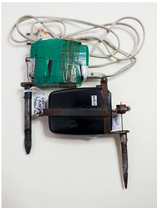
Fig. 15. These electrical razors have been rebuilt into tattoo machines and were often used in prisons. A prisoner with a bit of technical skill would easily be able to do this.
