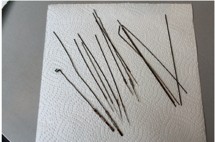
Fig. 13. Needles from the 1970s were mounted on spokes and hairpins.
