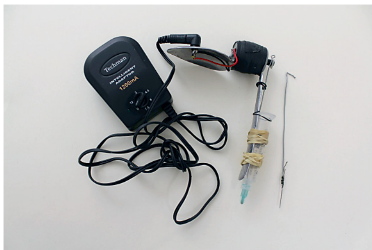
Fig. 16. This is a more recent prison machine. The engine is probably from a cassette player, and if you add to it a bit of scotch tape, a bent spoon, a ball-point pen and a sewing needle, you've got yourself a tattoo machine.
