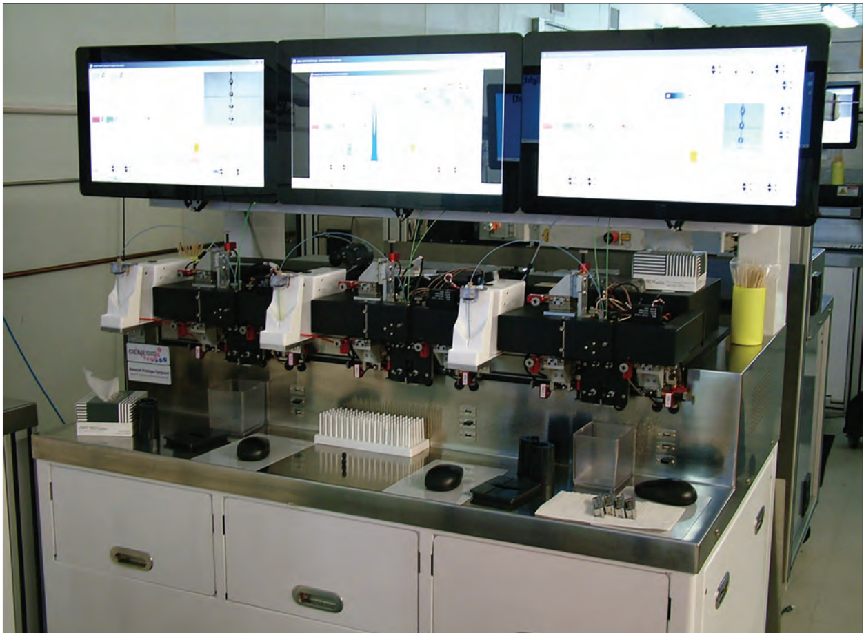
Figure 8.5: A state-of-the-art GENESIS III flow cytometer used for the sorting of sperm cells into X and Y populations. Photo courtesy KM Evans (Sexing Technologies), used with permission from ST Genetics.
