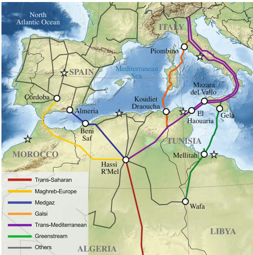
Fig. 3.17 The existing gas pipeline network between Europe and North Africa can be used to transport renewable gas from desert energy to Europe. The coloured and the grey lines indicate existing gas pipelines. The thin black lines are country borders [70]
