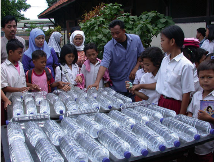
Fig. 2.8 Solar water disinfection in PET plastic beverage bottles kills most pathogenic germs (e.g. bacteria, viruses, protozoa and worms) by a combination of UV light irradiation and solar thermal temperature increase [91]
