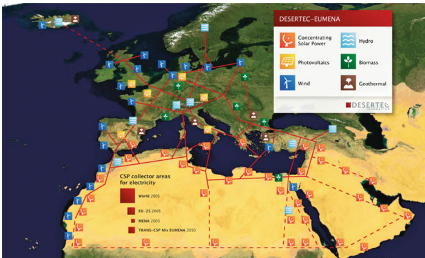
Fig. 3.10 The original DESERTEC concept suggests a HVDC transmission network to trade electricity between Europe and Middle East and North Africa (MENA). The dominating sources were Concentrated Solar Power stations in the deserts and wind power in the coastal areas, on- and offshore. In addition, all other renewable energy sources like hydro, PV, biogas, and geothermal energy were included [43]
