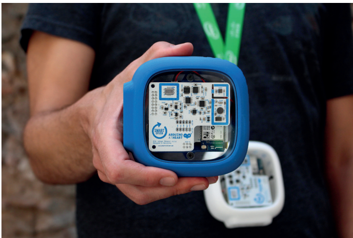
Fig. 16.2 The Smart Citizen Kit, a DIY and open source sensor. (Source: Smart Citizen team; Fab Lab Barcelona | IAAC and MID)
