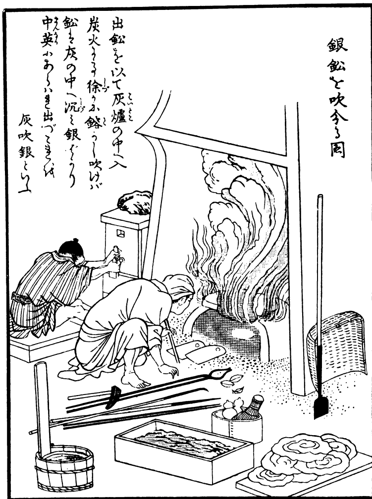
FIG. 27. The cupellation of argentiferous lead in Japan.
