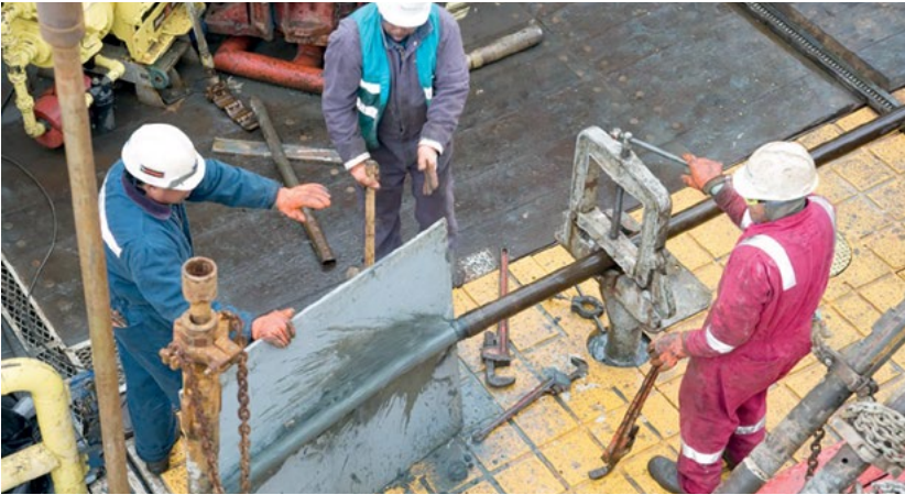
Figure 6.9. Drill core on deck. There was so much expanding gas in the sediment that it shot out of the core barrel when it arrived on deck
