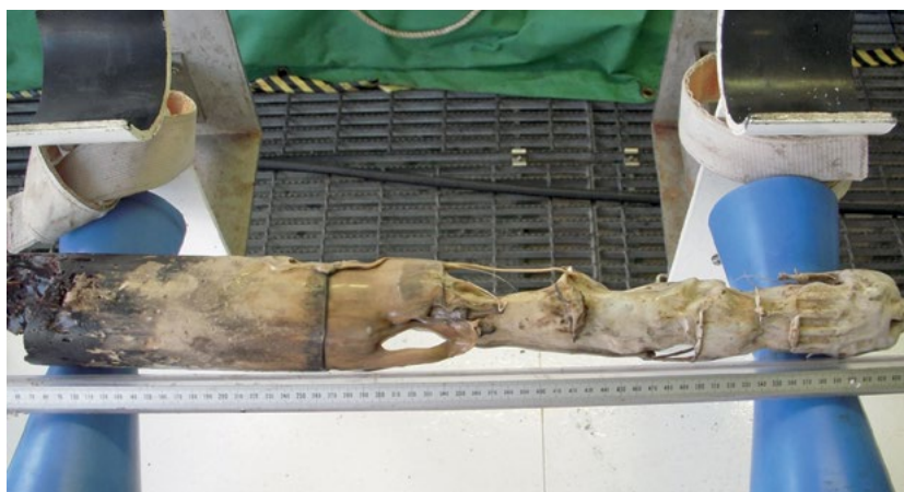
Figure 6.16. All that remained of a 9 m Perspex core liner after an early drilling attempt at our first site, melted by the very high temperature
