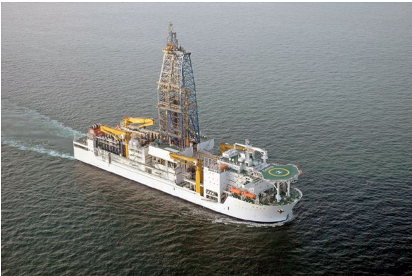
The Japanese deep-drilling vessel Chikyu at sea. It can core up to 4,000 m below the seabed and in areas where there is a potential danger of striking oil or gas
