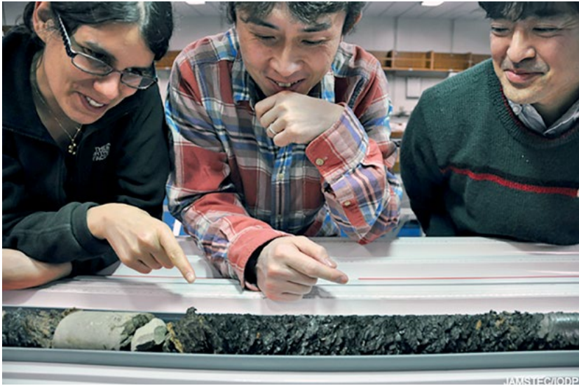
Figure 7.16. Drs Marianne Cronin and Kohtaro Ujiie and Professor Jim Mori (PI) examine core '17R', which sampled part of the plate boundary décollement between the Japan and Eurasian plates at the Expedition 343 site
