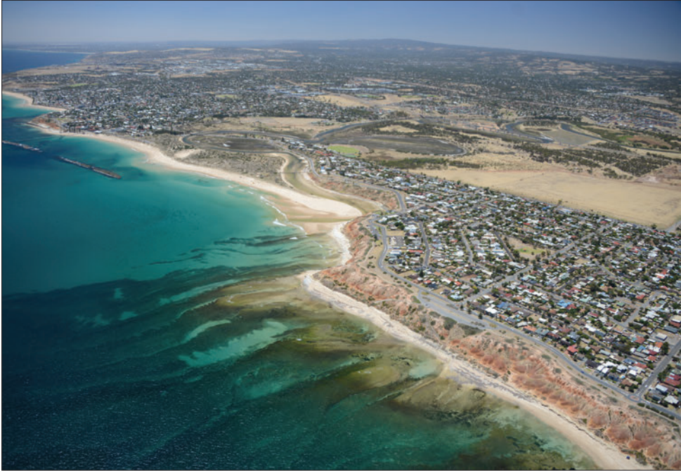
Figure 2.7 Onkaparinga Estuary and the spit, which is 2 km long and has diverted the river to the south against the cliffs. On the left of the photograph, the shore-parallel Noarlunga Reef protects the beach.
