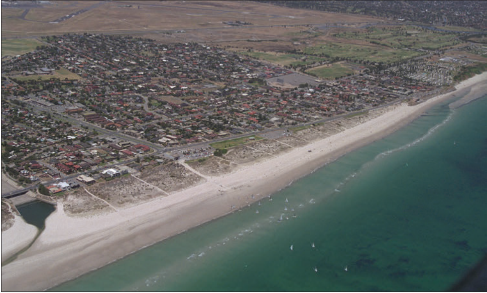
Figure 2.13 Torrens Outlet to West Beach, illustrating the extensive build-up of sand south (to the right of the photograph). The sand has been trapped partly because the outlet acts as a hydraulic groyne but also because of an extensive dune revegetation programme of native species.
