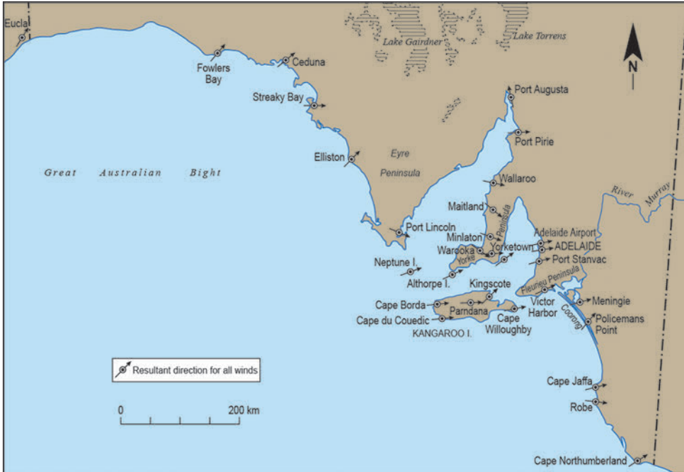
Figure 1.15 Resultants of sand-shifting winds along the South Australian coast, calculated using the Landsberg (1956) formula, which demonstrates the dominance of onshore southwesterly winds. 72
