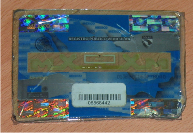
FIGURE 7. REPUVE RFID tag. Photo by Keith Guzik, © 2015.
