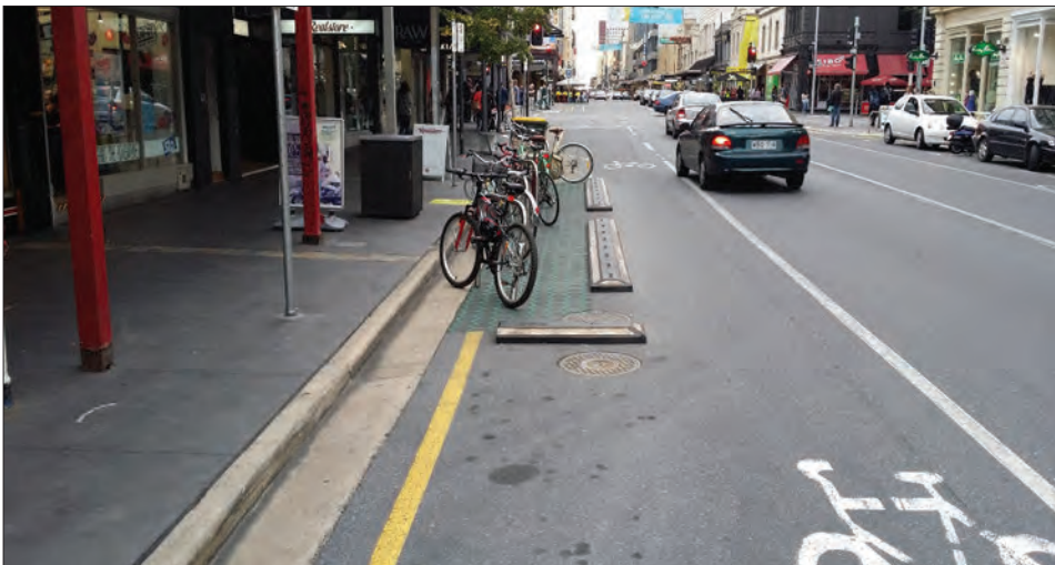
Figure 12.9: Reallocation of central city street space to bike parking and a cycle lane, Adelaide, South Australia. (Source: Author.)
