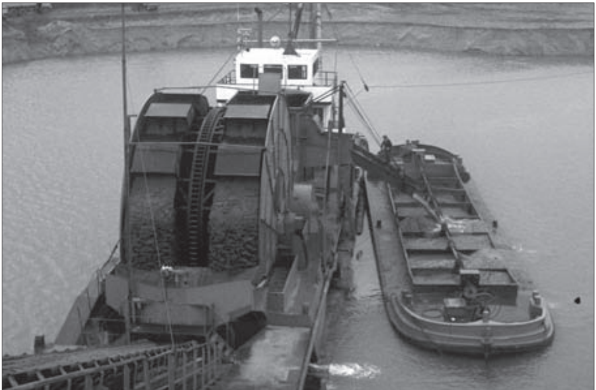
Fig. 7.3. Dredging operations in the dredge-pit in 'de Kesselsche Waarden' at Kessel in 1985. General view (a) and the separation of sand and gravel (b). Photographs by the author.
