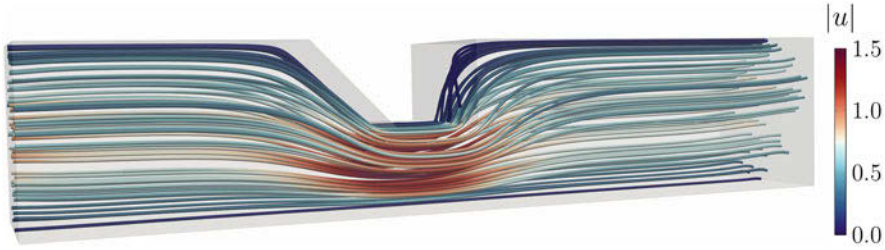
Fig. 9 Velocity streamlines for the non-linear generalized Newtonian Stokes problem
