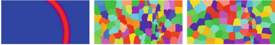
Fig. 8 Left: workload distribution for a selected time step of the 2D shock scenario, red indicates 4 times increased workload; Center: Resulting partitioning for 96 processes with ParMetis, colors represent individual partitions; Right: Resulting partitioning with Diffusion
