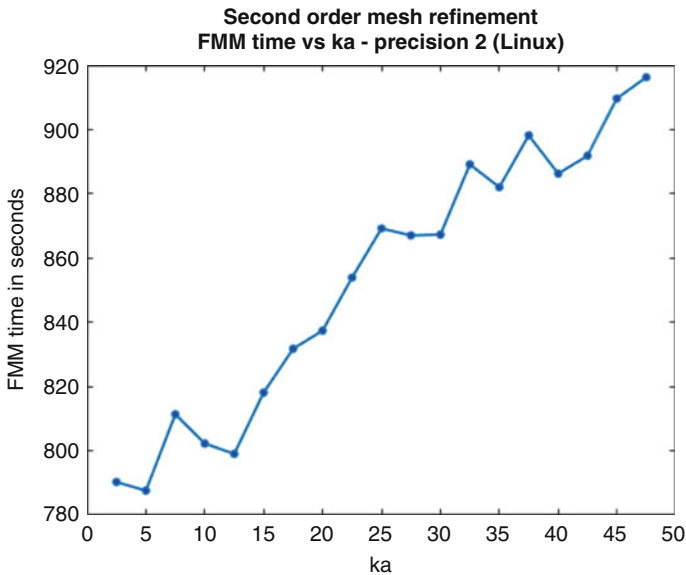
Fig. 36 Average FMM runtime for the doubly refined models in MATLAB on Linux is plotted with respect to values of ka . The demanded precision is six digits accuracy
