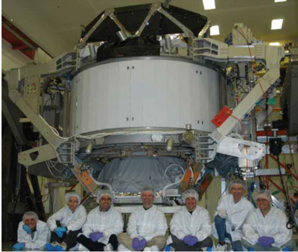
Fig. 18.16 The AMS-02 spectrometer during its integration at CERN in 2009 in the final flight configuration with the permanent magnet
