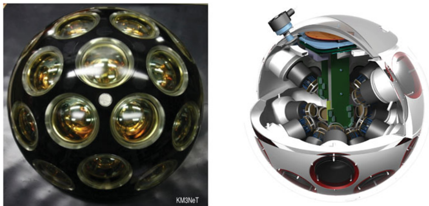
Fig. 17.18 View and a cross-sectional drawing of a KM3NeT-DOM with its 31 small PMs inside [64]
