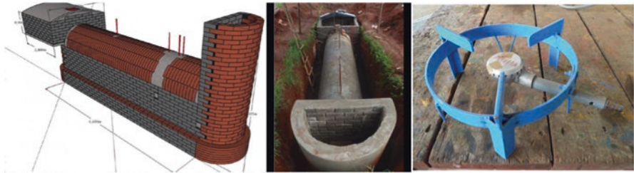
Fig. 5.3 The biogas system analysed in the present work comprises a small-scale biogas digester (left and centre) and a LOTUS biogas burner (right). (Source: Schrecker 2014)
