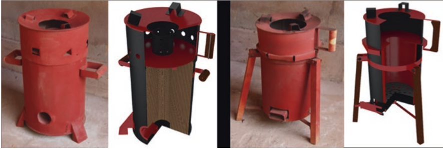
Fig. 5.5 The microgasifier stoves analysed in the present work comprise an improved sawdust stove (left) and a TLUD stove (right). (Sketches and photographs by D. Fröhlich)
