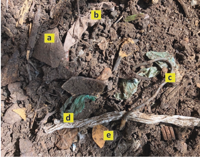
Fig. 4.3 A sample of MSW-based compost just before sieving. This compost contained non-biodegradable materials such as (a) pericarps of fruits that are hard to decompose, (b) textile materials, (c) wires, (d) polythene, (e) leather, etc. that would end up in a rejected pile after sieving. (Photo credit: Dandeniya)
