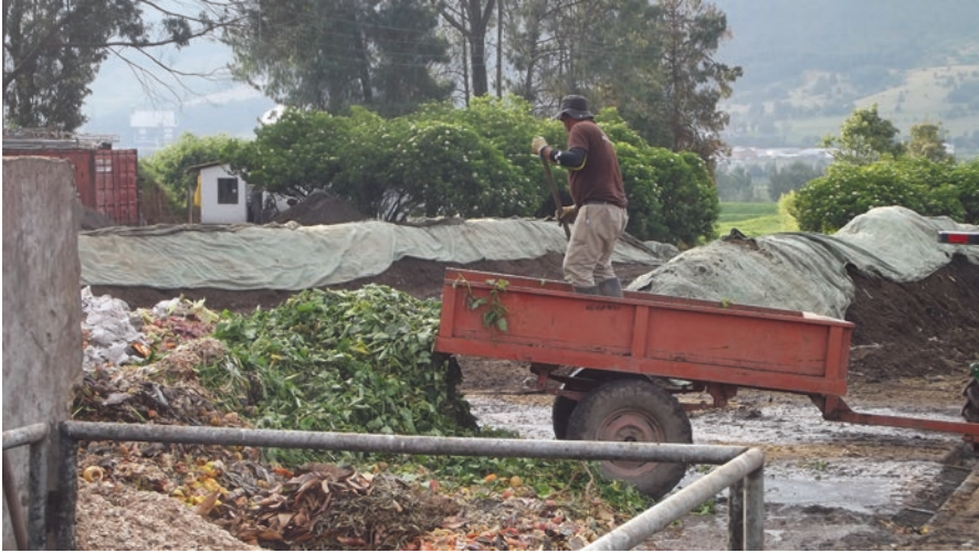
Fig. 2.7 Composting in operation at the IBICOL SAS facility as organic waste received is being unloaded. After 24 h, this waste is transferred to the piles seen in the background for the next stage of processing (Photo taken by the authors in November 2018 with courtesy of the General Manager of the Facility, Mr. Francisco Pradilla)
