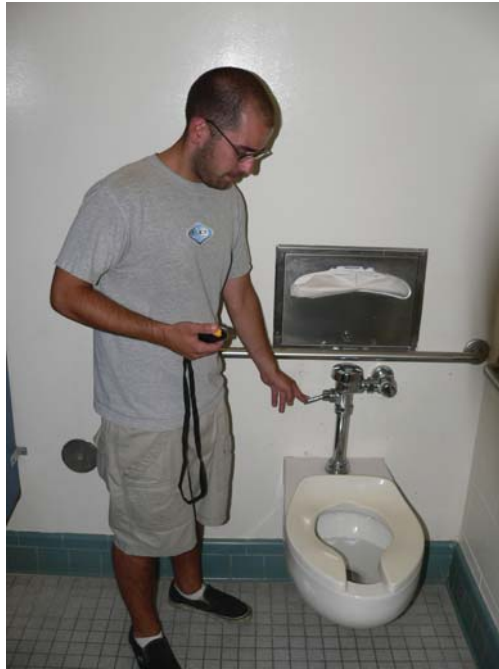
Figure 6.6 Conducting a commercial water audit and checking toilet flush volume. Source: Maddaus Water Management (2005).
