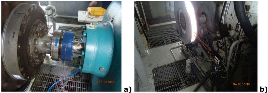
Figure 2. Torsional vib. instrumentation a) strain gauges at the coupling spacer and gearbox input shafts and b) laser vibrometer, beams highlighted.
