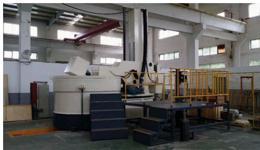
Figure 3. The photo of the high-speed rotating test rig.
