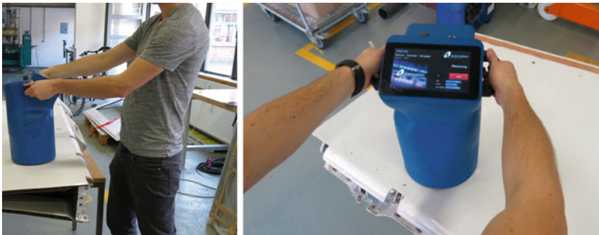
Fig. 6.3 HANOB demonstration setup operated for the inspection of a wing flap from Airbus Germany
