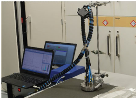
Fig. 5.20 The e-nose desorber device taking measurements on the CFRP Panel 1 within the production user case during the full-scale demonstration event
