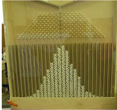
Fig. B.7 The binomial distribution as a sum of Bernoulli random variables. At each step, every steel ball moves to the left or to the right with equal probabilities, i.e., by 2X_n - 1 where X_n is Bernoulli 0.5. The position after N steps is Y = \sum_{n=1}^N (2X_n - 1) = 2B(N, 0.5) - N . After M balls, the stacks show approximately the values of M \times P(Y = y) for integer y 's
