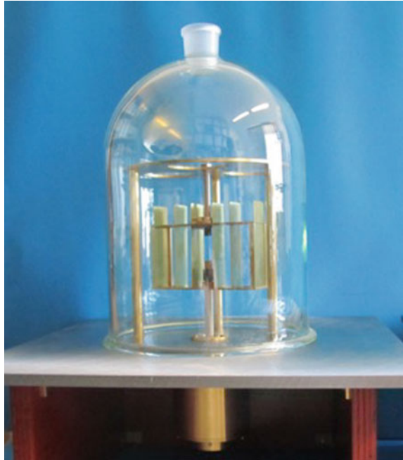
Fig. 11 Reconstructed apparatus to measure the Maxwell velocity distribution (without vacuum pumps and diagnostics)
