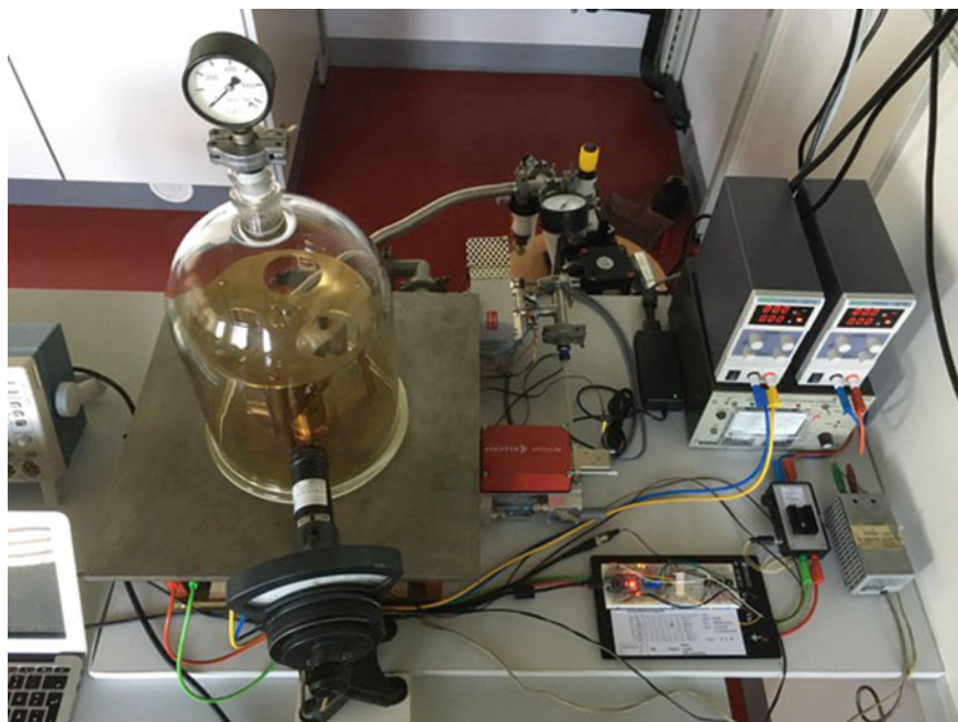
Fig. 14 The final experimental setup of the Otto Stern experiment in 2019: In the center: glass recipient with pressure gauge on an iron plate. Inside, the fixed frame with the rotating slit system is visible. On the right: parts of the vacuum system with backing pump (red, in front) and turbo-molecular pump (rear). In the foreground in front of the glass bell stands the pyrometer (“Pyropto”, Hartmann & Braun ® ) for temperature measurement. Right front: PID controller for speed control on breadboard with an ARDUINO ® controller. Rear right: controllable DC power supplies for the motor and the heating wire. Below is the vacuum measuring device with the vacuum display. The Pirani and Penning sensors (Balzers ® ) are positioned under the base plate and are not visible. On the left: Laptop for setting and logging the rotation speed during the measurement
