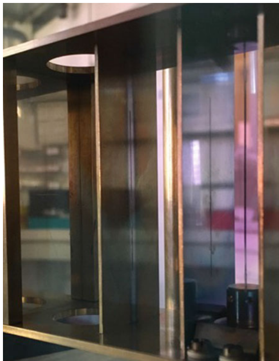
Fig. 18 The slit system with the detector plate after the experiment. On the right is the platinum wire; on the left, next to it, is the first slit aperture, which is completely covered with silver. To the left of it is the second slit aperture on which one can clearly see the “shadow” of the first slit aperture. On the far left, the detector plate is to be seen, on which a faint, brownish Ag line is just visible
