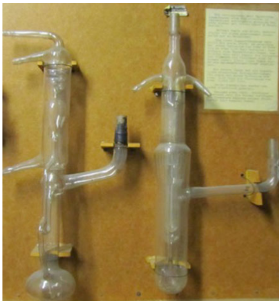
Fig. 5 Historic pumps used in the original SGE. Left the Volmer mercury diffusion pump, right the Gaede diffusion rough pump [photo HSB]
