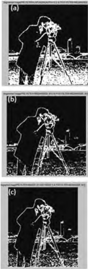
Figure 29.5 Output of Median post-filtered segmented image applied on the image which is pre-filtered using the (a) Laplacian filter, (b) median filter, (c) min filter.
