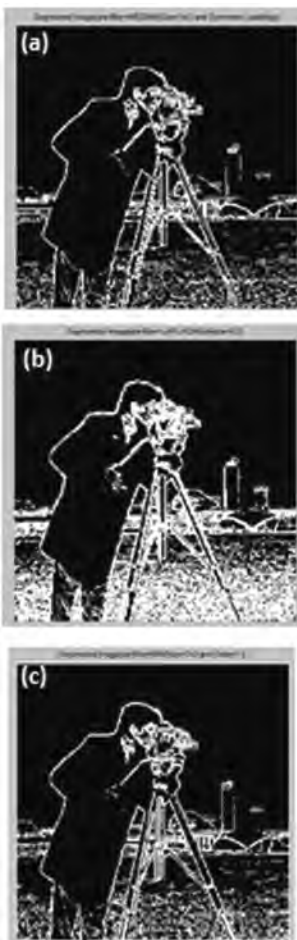
Figure 29.4 Output of Laplacian post-filtered segmented image applied on the image which is pre-filtered using the (a) Laplacian filter, (b) median filter, (c) min filter.
