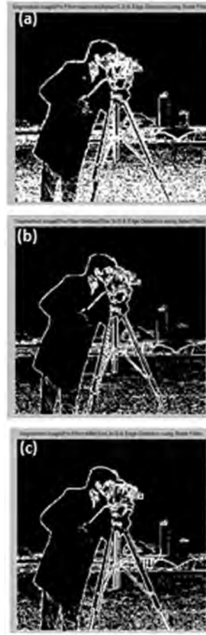
Figure 29.6 Output of Sobel post-filtered segmented image applied on the image which is pre-filtered using the (a) Laplacian filter, (b) median filter, (c) min filter.
