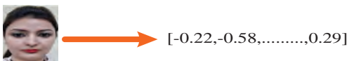
Figure 50.6 Generation of the 128-d real-valued number feature vector of each training image in the dataset.
