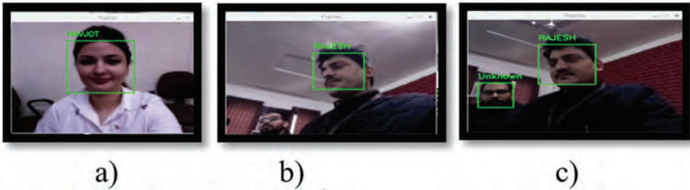
Figure 50.9 Face recognition results. (a) Face recognized as Navjot. (b) Face recognized as Rajesh. (c) Unknown face detected.
