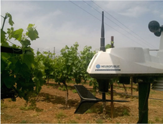
Fig. 15.3 NP's IoT agro-climatic station used in the pilot activities
