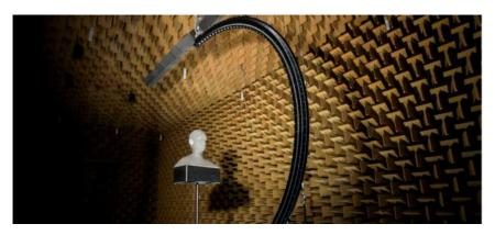
Figure 4.1.: Measurement setup of the arc and an artificial head on a rotating turn table at ITA, RWTH Aachen University.
