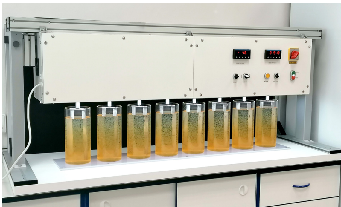
Figure 3.1 A paddle stirrer (jar tester) LMK 8 (Institute of Hydrodynamics of the Czech Academy of Sciences) with eight 2 L jars.
