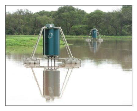
**Figure 5.20** Wind-powered slow mixers in a facultative pond of the sanitation cooperative SAGAUPAC, Santa Cruz, Bolivia. If properly employed, the slow mixers greatly reduces vertical stratification and hydraulic short circuiting.
