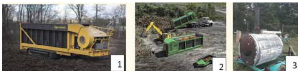
Figure 5. Representative mobile BC production systems: (1) carbonator 6050, (2) air burner fireboxes, and (3) cooker.
