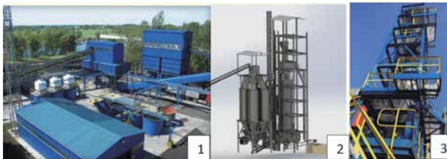
Figure 6. Representative continuous BC production systems: (1) Polchar production facility, GCS's (2) vertical retort process and (3) vertical retort.
