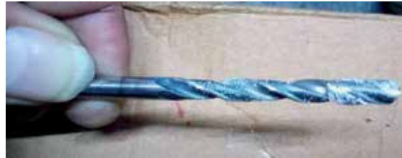
Figure 9. Adhesion of material to the drill bit.
