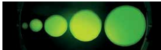
Figure 7. Roundness of holes produced by AWJ.
