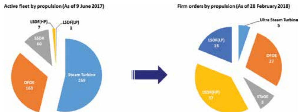
Figure 15. Development trends of propulsion system.
