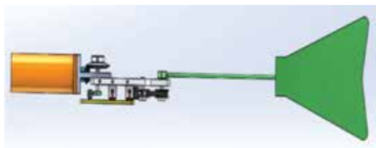
Figure 22. Caudal fin propulsion mechanism.
