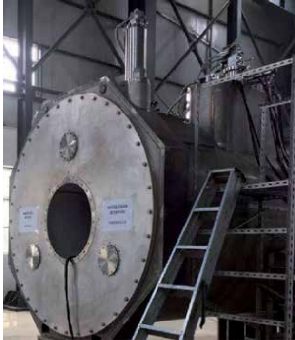
Figure 2. A 9.4 T superconducting magnet for whole-body MRI system.
