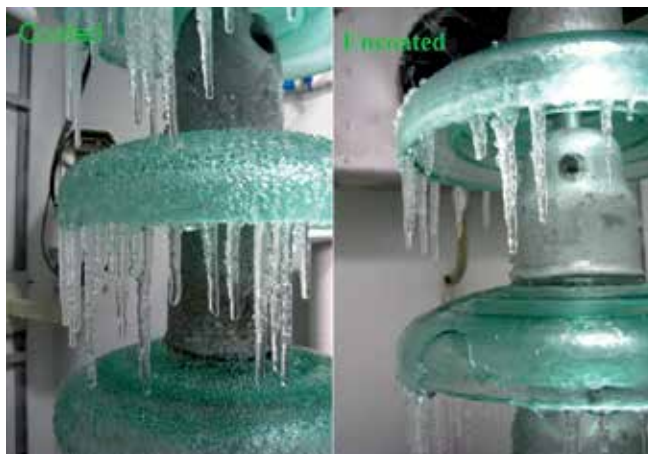
Figure 5. Comparison of the ice formation on the uncoated and superhydrophobic-coated insulators [5].
