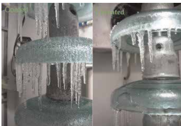
Figure 11. Comparison of the uncoated and superhydrophobic coated sample at -5^{\circ}\text{C} and high humidity [35].
