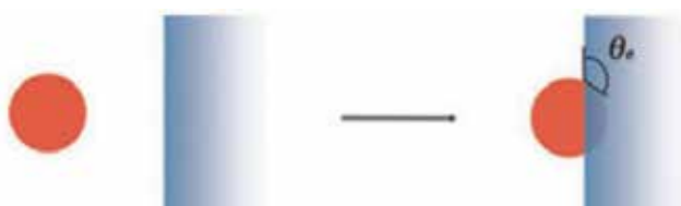
Figure 8. Schematic of the spherical particle that has moved from air into the water; the contact angle between the particle and water is shown [25].
