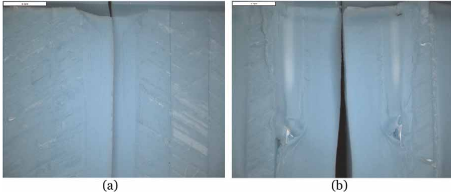
Figure 13. Corresponding fracture surfaces at 1 mm/s (a) 2VN-1sp and (b) 2VN-2sp weld configurations. A distinct welding defect is also shown in figure (b).
