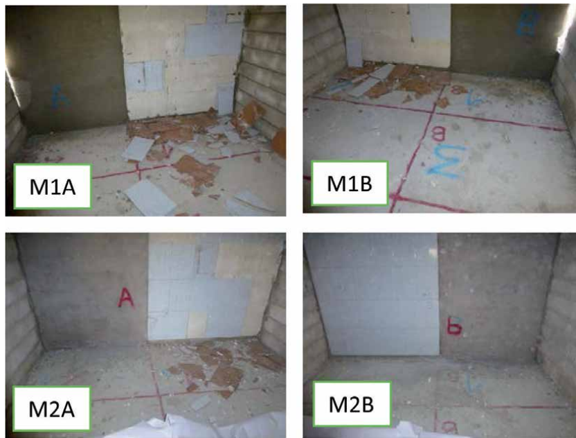
Figure 5. Fragments inside the boxes after the test.
