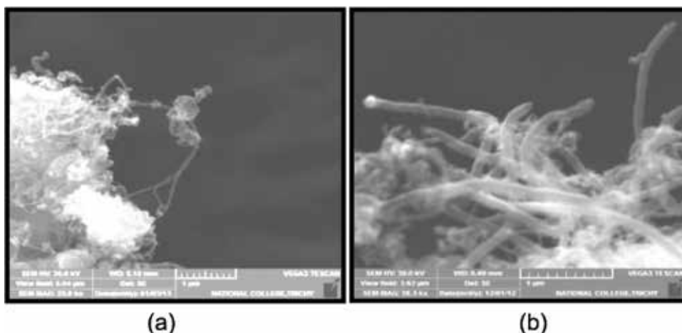
Figure 7. (a and b) SEM images of MWNTS grown at the flow rate of 10 and 30 mL.
