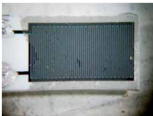
Figure 7. Functionalized nanotubes self-assembled in dense arrays (monolayers), covering without empty space the whole surfaces of the finger-shaped electrode device.
