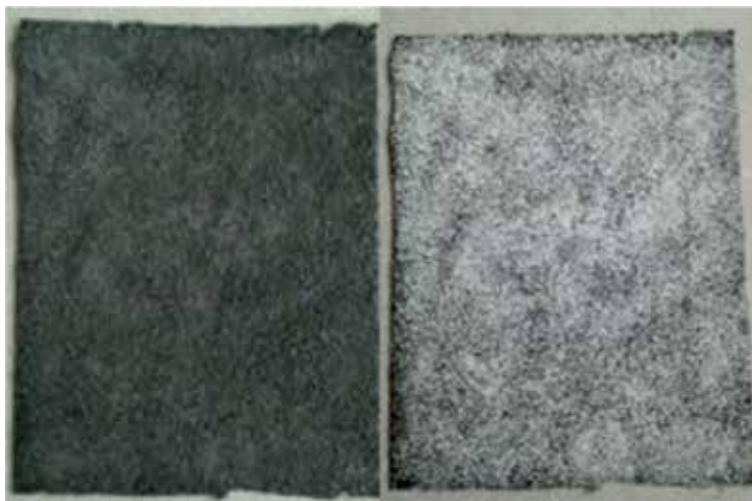
Figure 9. Thermochromic polymer particles can be used to coat a surface such as asphalt shingles to allow color changes to the surface-applied particles based on temperature. Source: [11].
