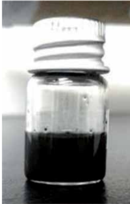
Figure 10. A suspension of CNT that can be used as a coating, paint or adhesive when mixed in production with an appropriate carrier material. Source: [11].
