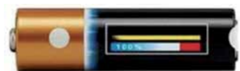
Figure 4. Smart particles provide a power meter directly on the side of a battery. Source: [11].
