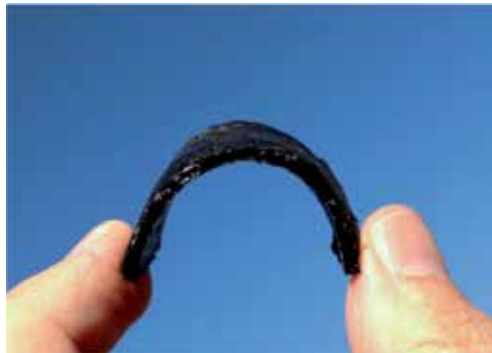
Figure 12. Smart damping adhesives can be formed as pads, gaskets, seals, o-rings or other three dimensional shapes. Source: [11].
