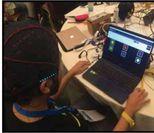
Figure 1. Calibration of the EEG experiment using the g.Unicorn EEG cap for a P300-based BCI.
