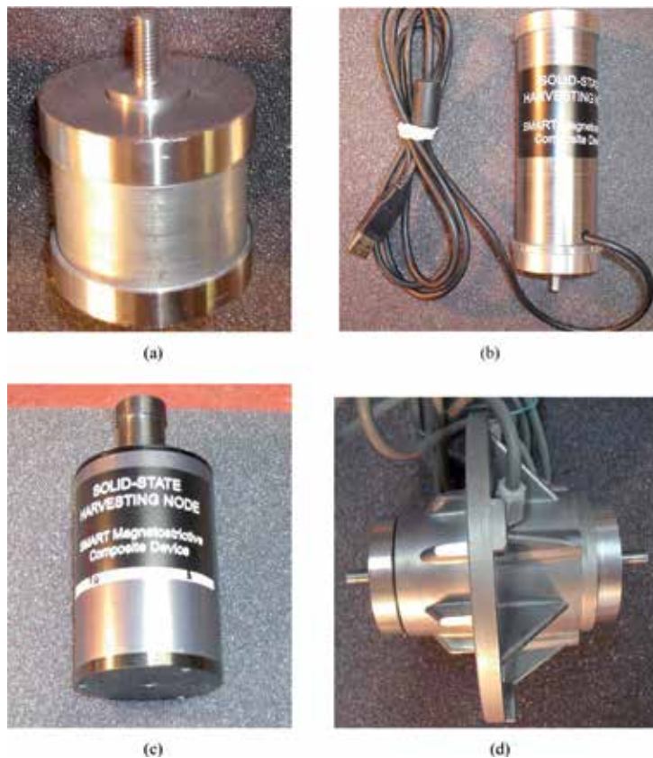
Figure 9. A view of prototypes developed in the Laboratory of Dynamics WRUT (a) and (d) low power harvesters, (b) high power harvester, (c) “Tactical grade” type harvester.
