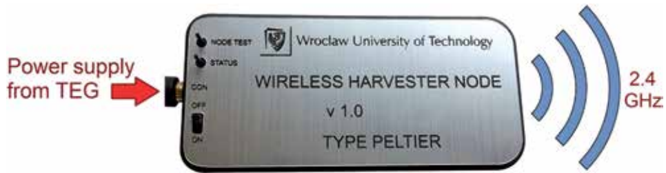
Figure 20. View of a single electronic wireless node powered from a harvesting source.
