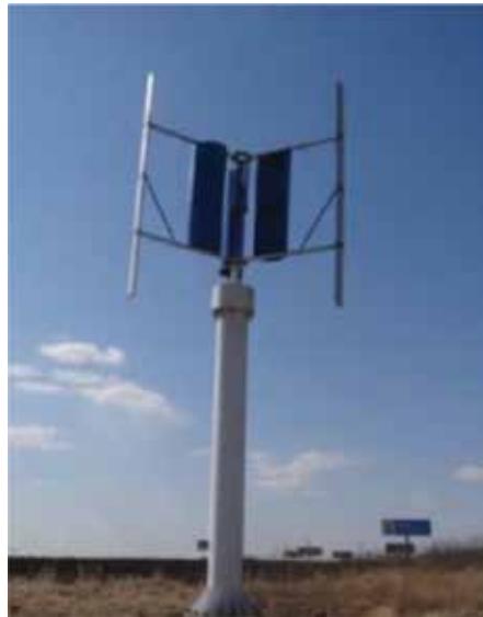
Figure 11. A prototype SB-VAWT for field test in NEAU.
