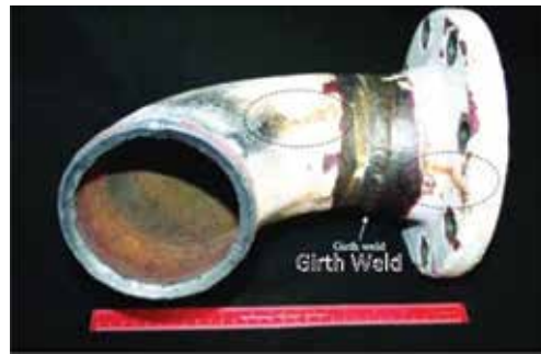
Figure 3. Photograph of cracked steel elbow welded to the flange [17].
