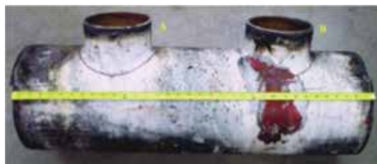
Figure 2. Locations of ethanol SCC near fillet welds used to make the branch connections to piping B [17].
