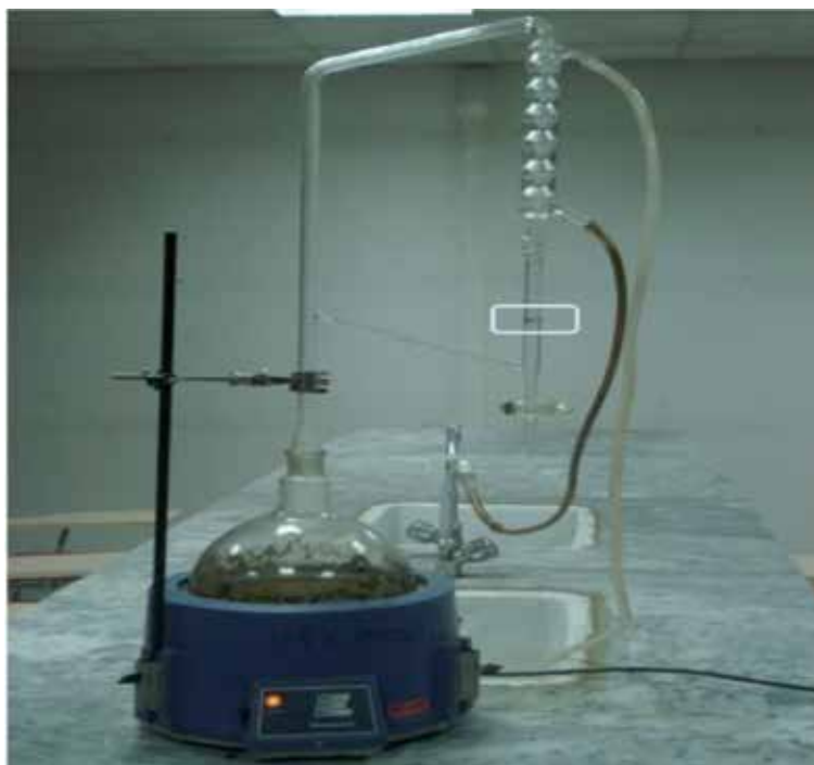
Figure 2. Hydrodistillation apparatus used for the extraction of essential oils.
