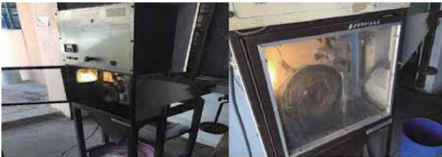
Figure 4. Abrasion test in progress.
